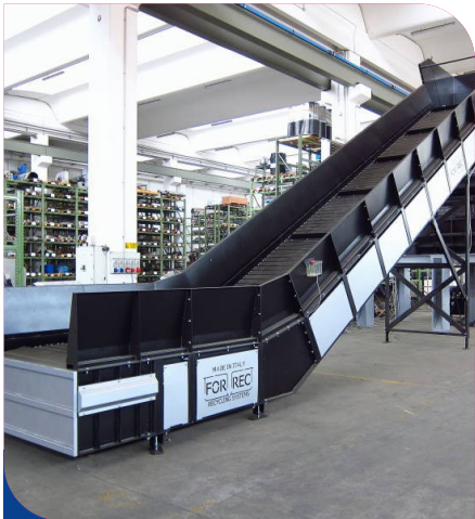
Metal apron conveyors, also available with rubber-covered plates and reinforced sidewalls, are designed to transport materials throughout the processing line.
