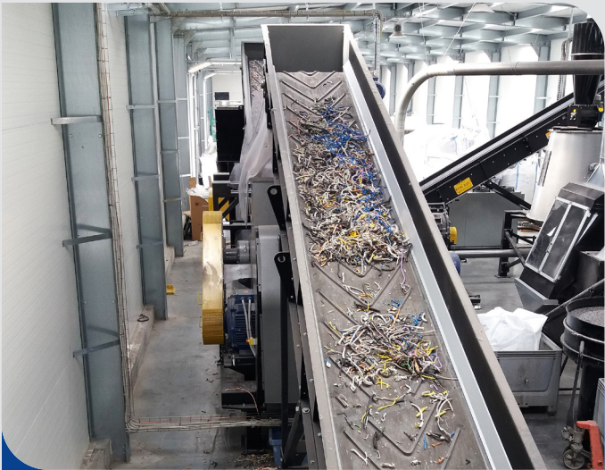
Automatic grinding and separation plant
