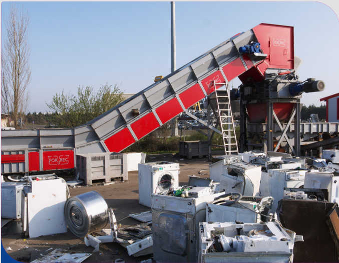
Automatic grinding and separation plant
