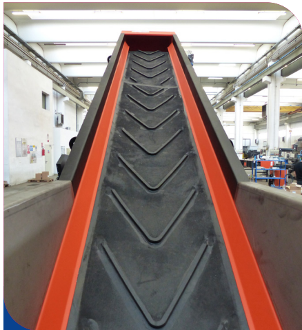
Rubber or PVC belt conveyors can be equipped with cleats, anti-drift guides, and containment sidewalls to ensure controlled material handling.
