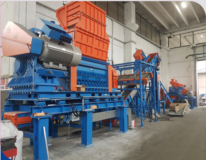
Automatic grinding and separation plant
