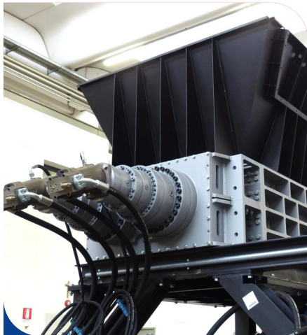
Counter-rotating shaft shredders suitable for the volume reduction of solid waste with partial control over output particle size.
