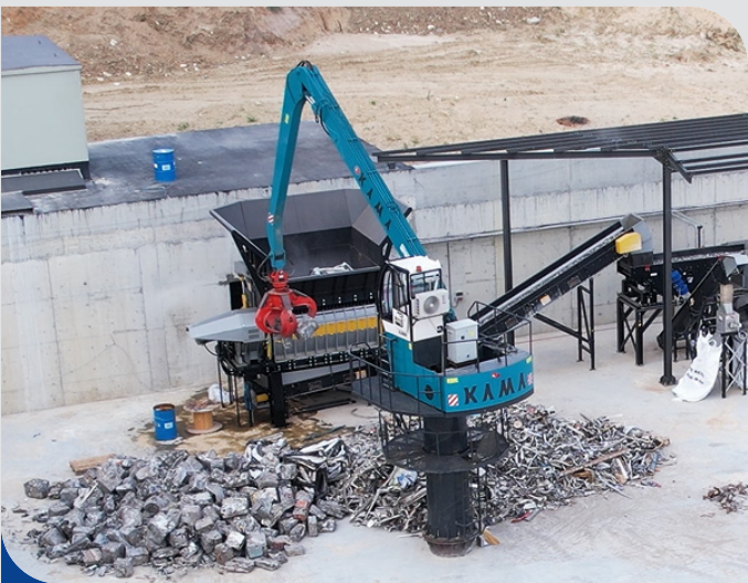
Automatic Grinding and Separation Plant
